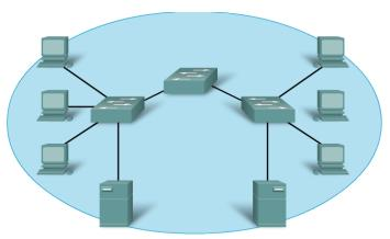
All devices in this network are connected in one broadcast domain when the switch is set to the factory default settings. Since switches forward broadcasts by default, broadcasts are processed by all devices in this network.
