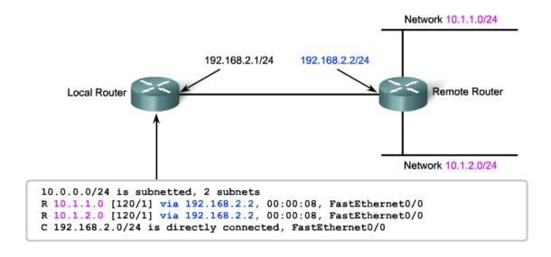
This is the routing table output of Local Router when the "show ip route" is issued.
